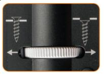
Before fastening on the deck top, drive a few screws into a scrap piece of material and adjust the depth set dial accordingly. For Edge screws, sink them 1/8-1/4 in below the surface of the deck board.
