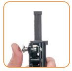
Insert the Face nose piece. It will lock into place.
